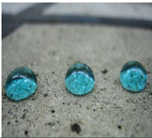
Concrete treated with API-WP40
